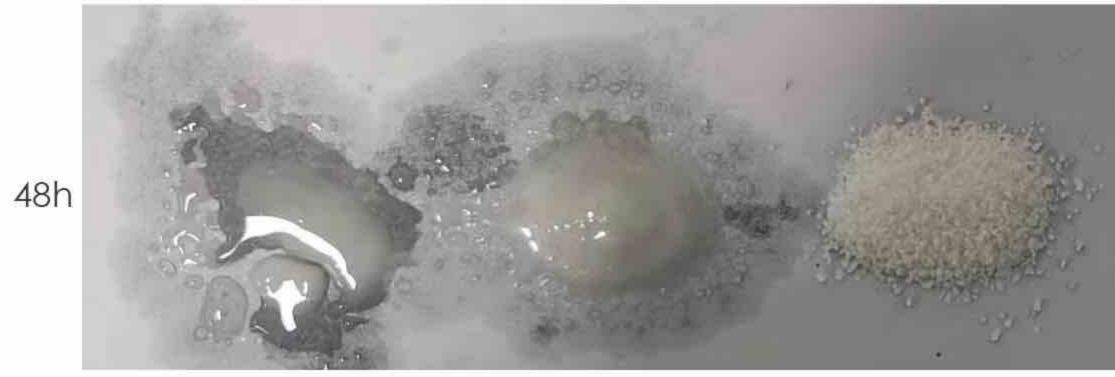
Comparison of 48h moisture-proof effect (Raw material: left Competitor: middle HSF SoliPro® Moisture-proof particles: right) L-carnitine remains stable at 25°C/50% for 48h after embedding, and has good moisture-proof effect.
